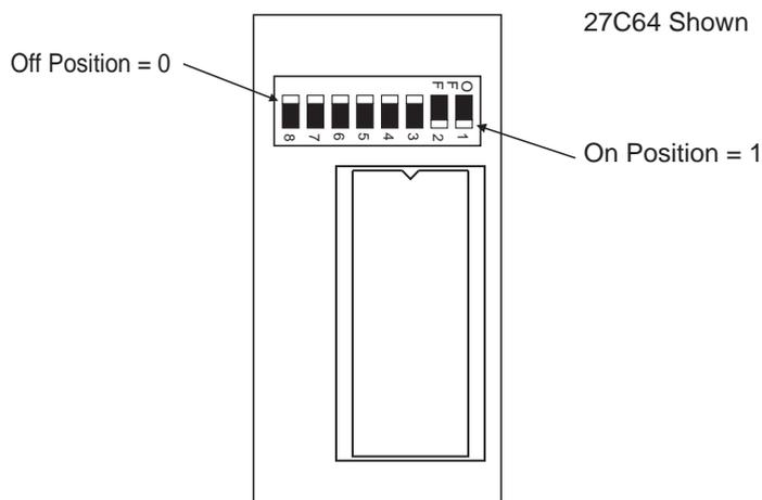
Figure 3.1 Channel DIP Switch Setting
